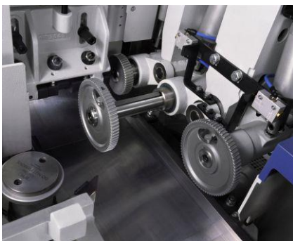
Extension of the pendulum arbor opposite the left spindles to 150 mm
