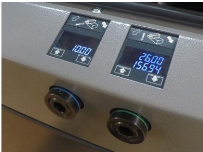
Radial CNC-controlled adjustment and positioning of tool holders in combination with Memory - Function or the PowerCom.
